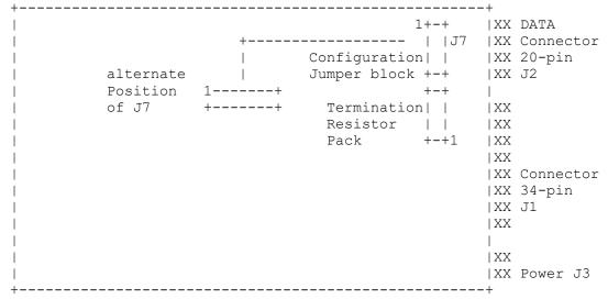
Alternate Location On Drive PC Board of the User Configuration Jumper. Note position of Pin 1 on both configurations. Jumper blocks in either position are identical in function.
