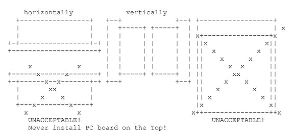
The drive may be mounted horizontally with the PC board down or on either side. Mounting vertically on either end is a prohibited orientation.
